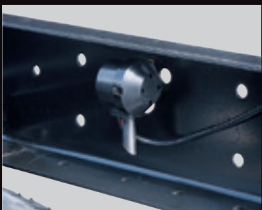
Reverse warning buzzer (option) Sounds to warn bystanders when truck is backing up
