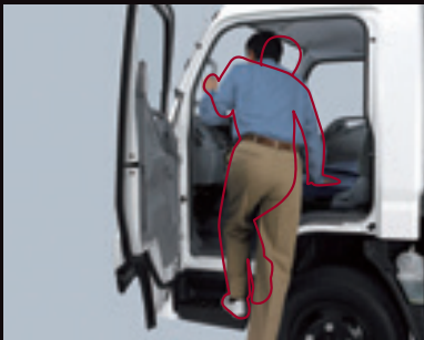
No need to bow The tall roof lets driver and riders get in and out in nearly standing position.
