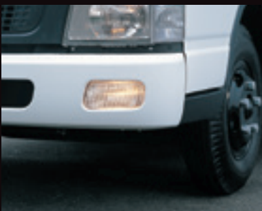
Fog lamps (option) For greater driving safety when visibility is poor
