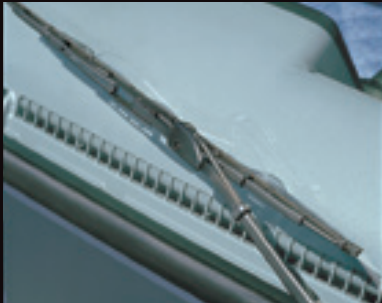
Wipers with integrated washer nozzles Nozzles moving with windshield wipers spray entire window. The result? Better cleaning.
