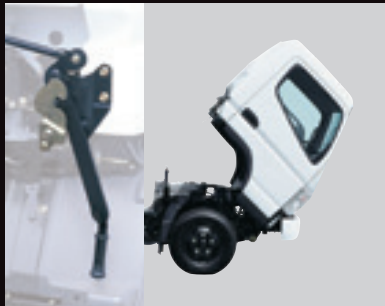
Passenger-side cab tilt lever Allows roadside tilting without standing in traffic.
